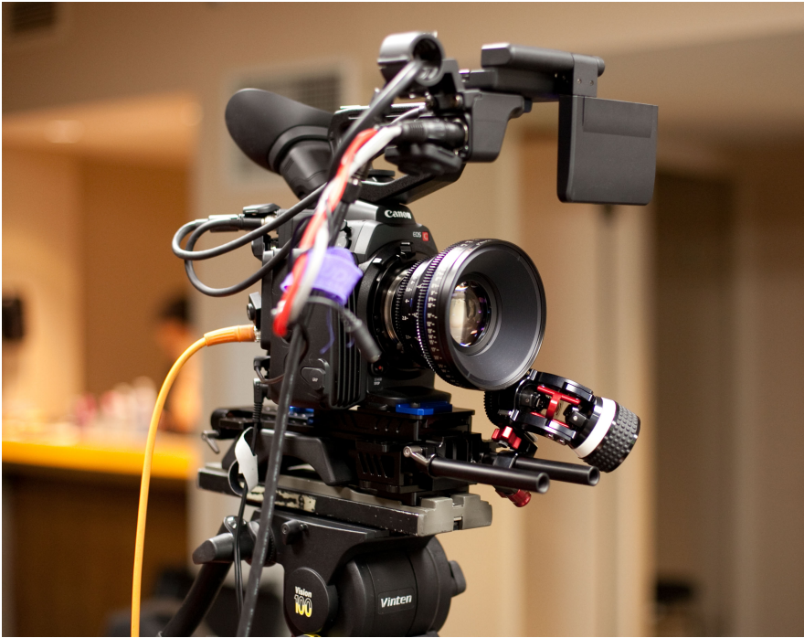
Figure 7: The Canon C500 digital cinematography camera. This large sensor camera is an excellent choice for on-location interviews and b-roll.
